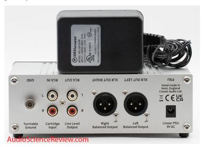
I like balanced output as audio gear has its only ground loops which we don't want to add the heap that phono stage may bring. As such, all of my testing was done using that output.
