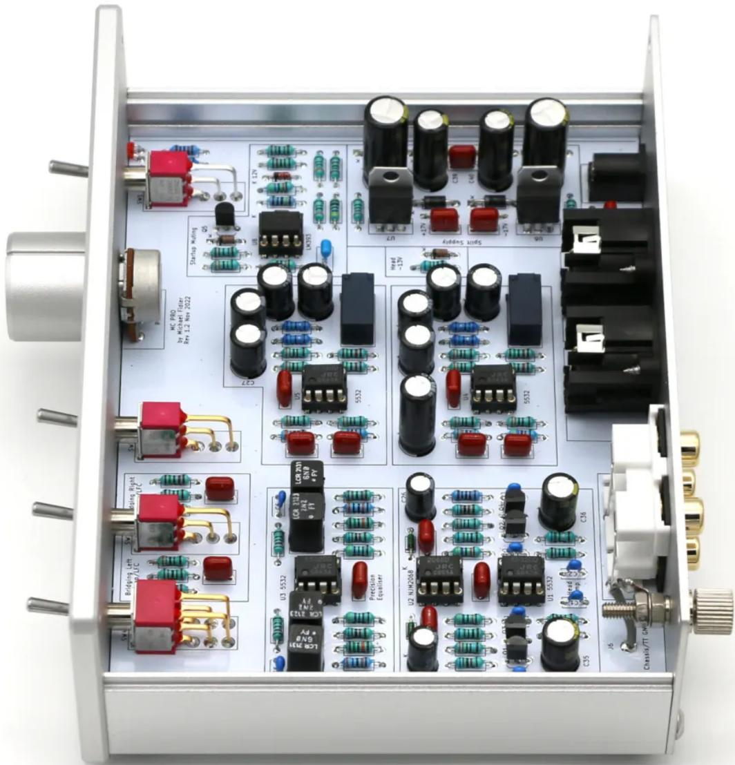
The toggle switches are made especially for Classic Audio and are rated for 50,000 cycles (as opposed to a more typical 10,000 cycles). They have a satisfying mechanical ‘clunk’ in operation and feel reassuringly stout. As much as I am a fan, proponent and even developer of microcontroller interfaces, there is something extremely satisfying about this strictly analogue, no-frills interface.
