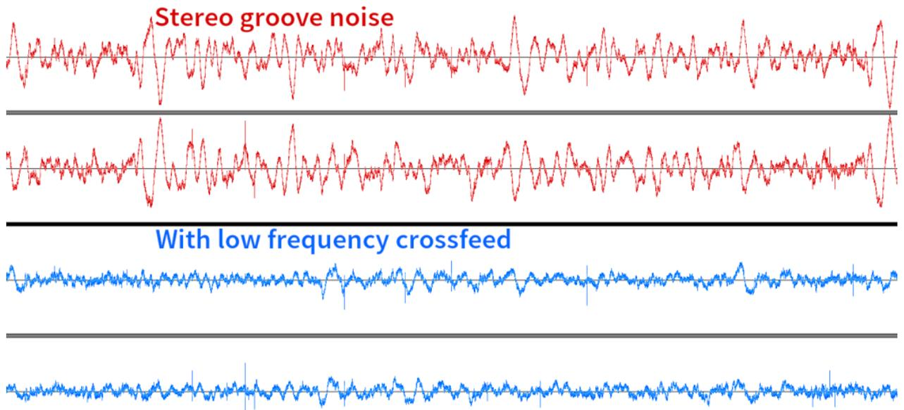
These noises exist on both channels and through headphones especially can be distracting, pulling the listener's attention to either side of the stereo field and to the rear of the three-dimensional image. Summing those frequencies to mono effectively puts them front and centre, removing the distraction and effectively hiding the unwanted noise beneath the desired musical content in the stereo field.
